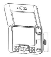
The replacement of batteries must take place within maximum time of one minute in conditions of flashing display.
