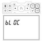
To unlock the keypad, press the **T1**, **T2** and **T3** keys again for 3 seconds and input, using the "\(\Delta\)" and "\(\black\)" keys, the protection password.
