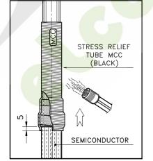
**4.6** Apply the **stress relief tube MCC** (black colour) in such a way to overlap the semiconductor for **5 mm**.
