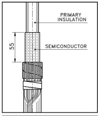
2.3 Remove the cable semiconductor (if necessary use appropriate tool) leaving exposed 55 mm from the outer jacket edge.
