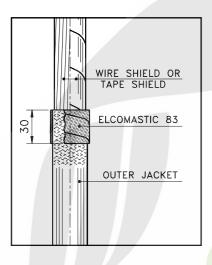
1.4 WARNING: The ELCOMASTIC 83 tape must be applied stretching up to reduce the original width to the half approximately and with 50% overlapped. Apply two halflapped layers of ELCOMASTIC 83 on the outer jacket edge for a tract of 30 mm starting from the edge.
