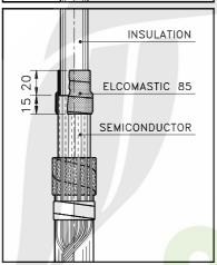
WARNING: The ELCOMASTIC 85 tape must be applied stretching up to reduce the original width to the half approximately and with 50% overlapped.
