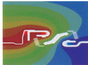
触头的电磁场分布 Distribution of magnetic field between contacts
