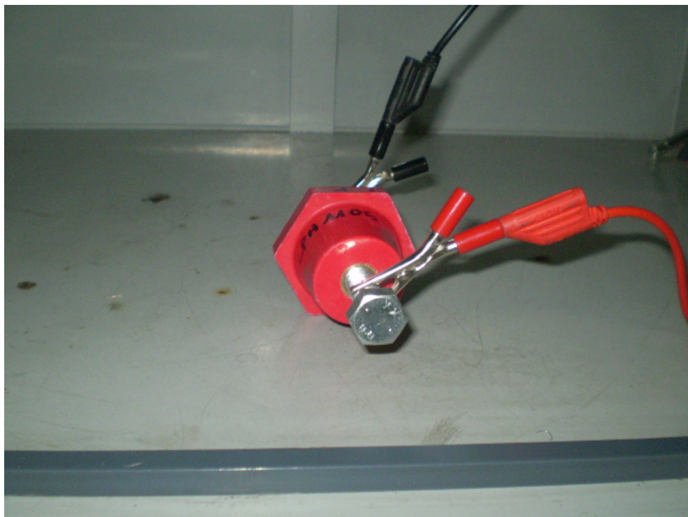
Fig. 2. - Set-up for dielectric test
