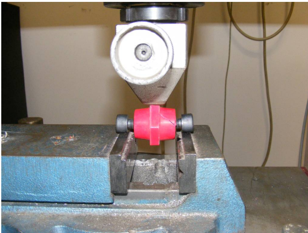
Fig. 4. - Set-up for flexion / cut test
